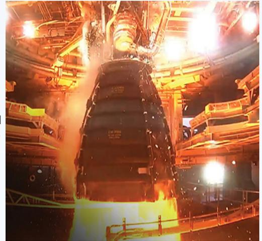
Abundant lighting is necessary for filming rocket engine testing, otherwise cameras will adjust to the brightness of the plume, obscuring the rest of the scene. Traditionally, metal halide bulbs have done the job.
